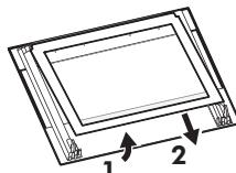
First lift carefully and then remove the glass panel. Pull the door trim to the front to remove it.
