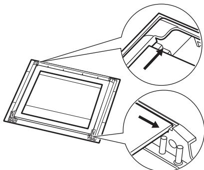
**⚠ Warning!** Danger of electrocution! Disconnect the fuse before you replace the lamp. The lamp and the lamp glass cover can be hot.
