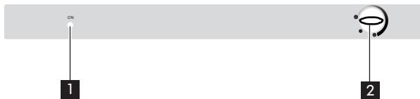
**1** The indicator light will glow to indicate the appliance is switched on.
