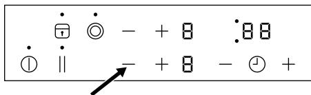
Touch + and — of a respective cooking zone simultaneously to deactivate the cooking zone. The settings will reverse to 0.
