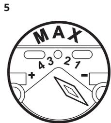
To adjust the released quantity of rinse aid, turn the selector between position 1 (lowest quantity) and position 4 (highest quantity).
