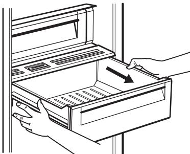
2. Lift the Low Temperature Compartment and pull out the glass cover with humidity control from underneath it.
