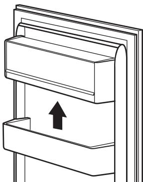
To permit storage of food packages of various sizes, the door balconies can be placed at different heights.
