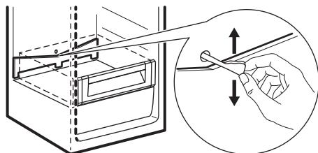
Frost is automatically eliminated from the evaporator of the refrigerator compartment every time the motor compressor stops, during normal use. The defrost water drains out through a trough into a special container at the back of the appliance, over the motor compressor, where it evaporates.
