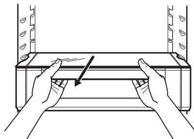
4. Tilt the module downwards to remove it from the refrigerator.
