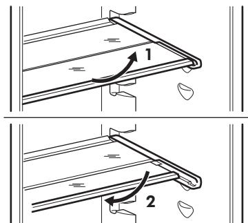
The walls of the refrigerator are equipped with a series of runners so that the shelves can be positioned as desired.
